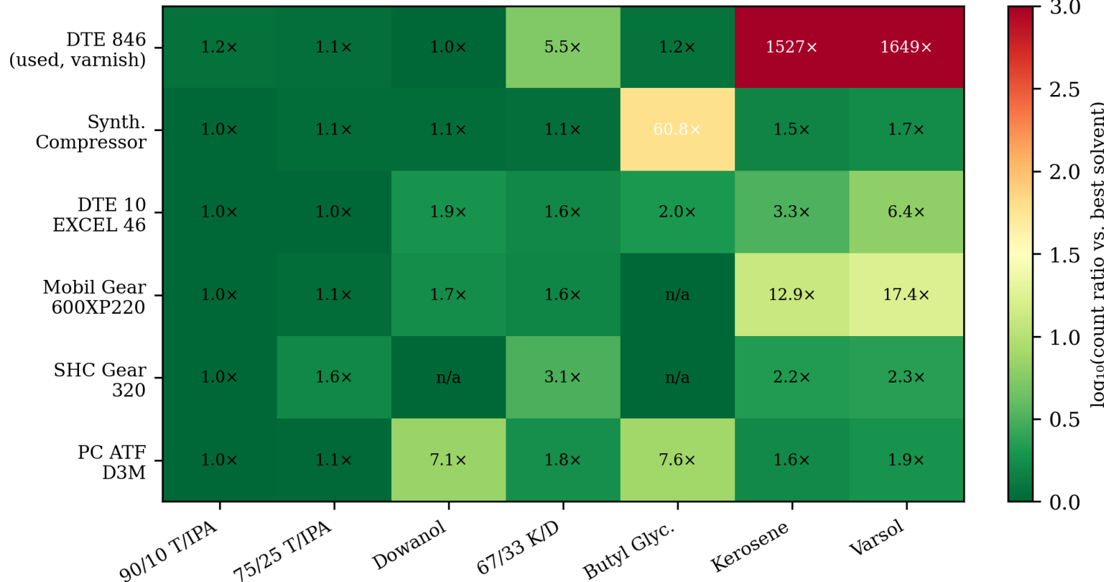
Relative >4 μm(c) count by sample × solvent. Values are mean(1:1, 1:2) divided by the lowest mean for that sample (=1×).
