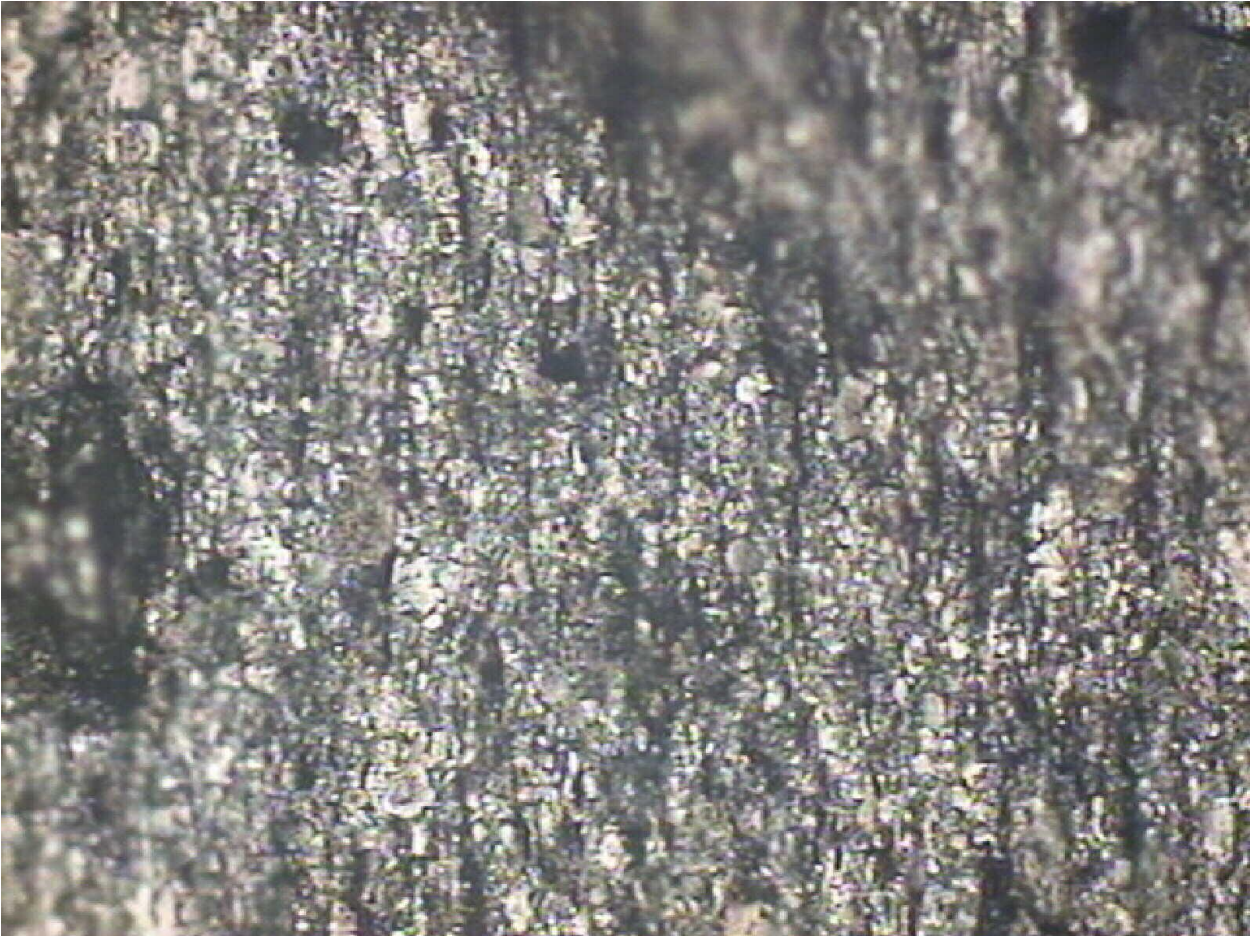
Figure C.2 – A ferrogram of the most current gearbox sample illustrating the high quantity of metal present in the oil (200x magnification, bichromatic light, sample prepared with 1:10 dilution).
